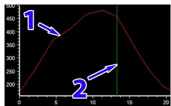
The red line (item 1 in the image) represents the arterial input. The green line on the arterial input graph (item 2) represents the current time point shown in the main viewport. The line is adjustable and when it is scrolled to a certain time point, the image in the main viewport shall be updated accordingly.
