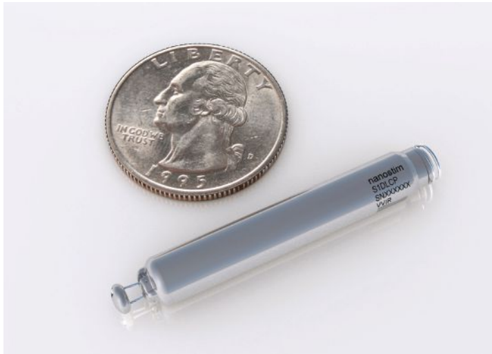
Small, leadless, wireless pacemakers like Abbott's Nanostim will likely replace larger, conventional pacemakers in select patients.
